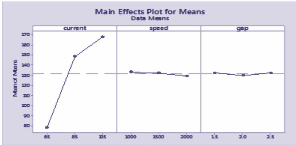
Fig.2. Main effect plot of S/N ratio Mean for higher MRR
